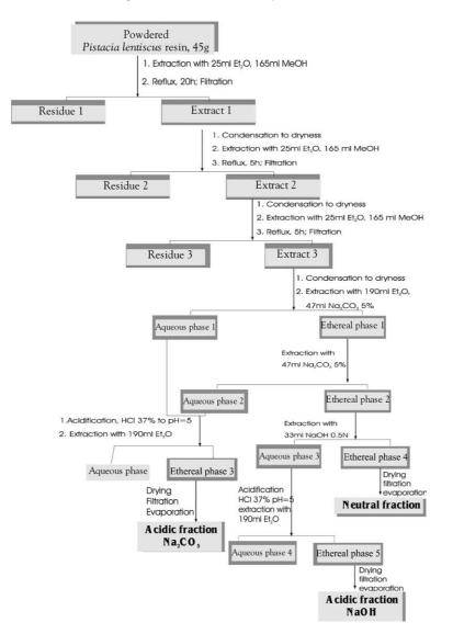
Fig. 2. Subfractionation of the resin Pistacia lentiscus var. Chia to a neutral fraction and two acidic ones (NaOH and Na<sub>2</sub>CO<sub>3</sub>).
